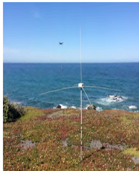
Figure 1: Antenna pattern from drone in red and blue plotted overtop transponder pattern (left) and drone flying in front of SeaSonde receive antenna (right)
