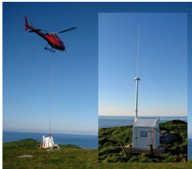
Fig. 1 Photos of self-contained SeaSonde HF radar being helicopter-deployed in Finnmark region of northern Norway during September 2010, during NOFO emergency-response exercise. Radar antenna is mounted alongside the weatherproof container and portable generator powers the system for up to a week
