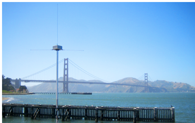
Figure 3. The 42 MHz SeaSonde antenna located at Crissy Field.
