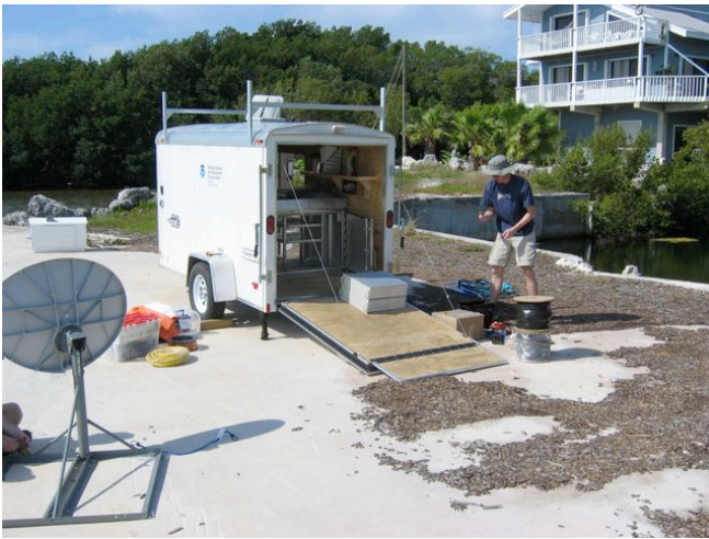
Figure 3. Mobile SeaSonde developed by NOAA CO-OPS being deployed in Key Largo, FL, USA.
