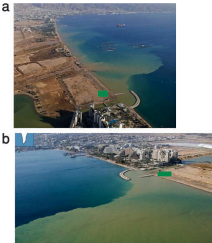
FIG. 7. Barrier to mixing as seen by aerial photographs showing that the sediments do not mix beyond the barrier that was calculated from the currents observed by the HF radar. (a) Taken from the northwestern corner of the gulf toward southeast on 3 Feb 2006. (b) Taken from inside the gulf facing northwest on 5 Feb, two days after the flood. The green rectangle in Fig. 4a and in this figure mark the same location. (Photos by Dubi Tal, Albatross Photography.)
