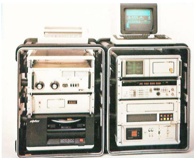
Figure 5. Photo of NOAA CODAR transmitter, receiver, DEC mini-computer, tape drive, and electronic test equipment -- vintage 1975.
