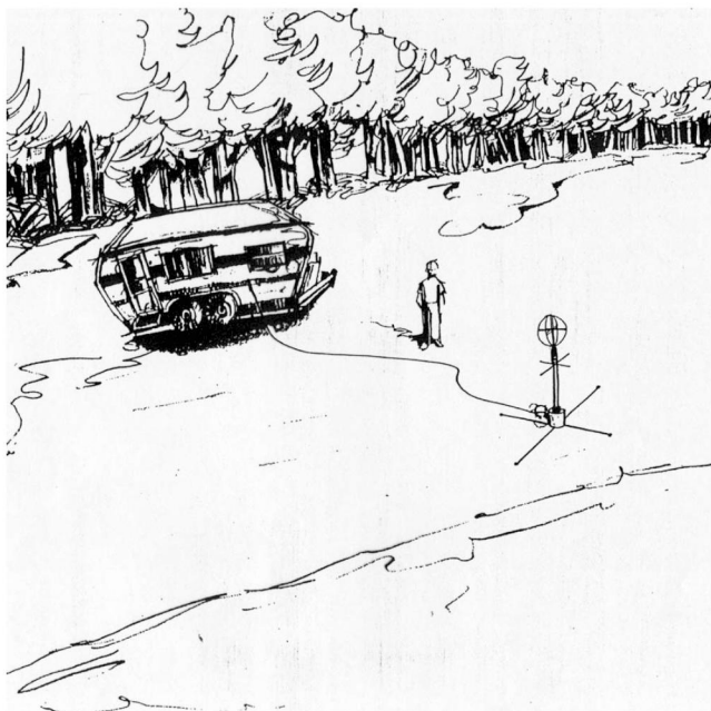
Figure 2. Sketch of DF antenna proposed to NOAA to replace phased array.
