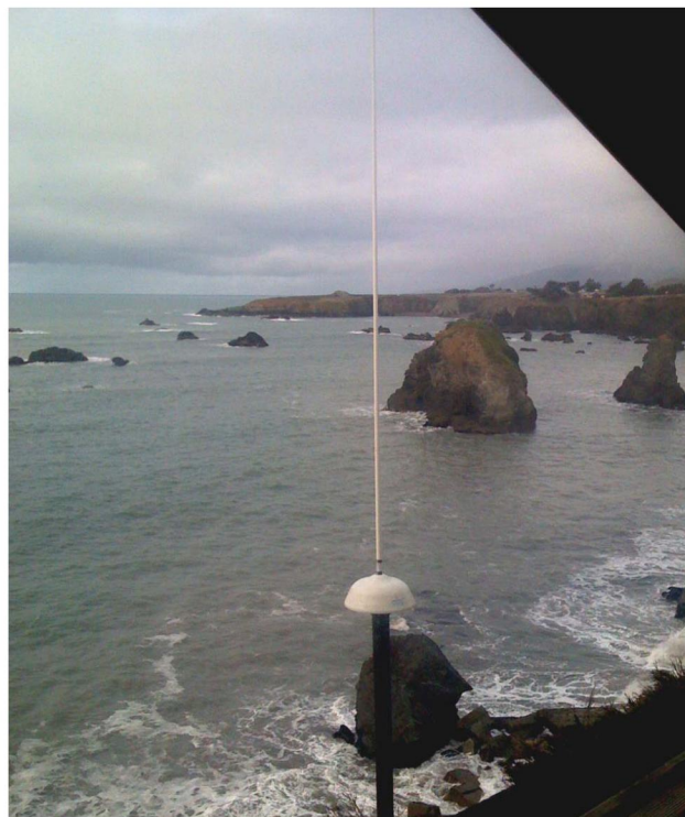
Figure 7. Latest SeaSonde crossed-loop/dipole antenna from 4 to 50 MHz.
