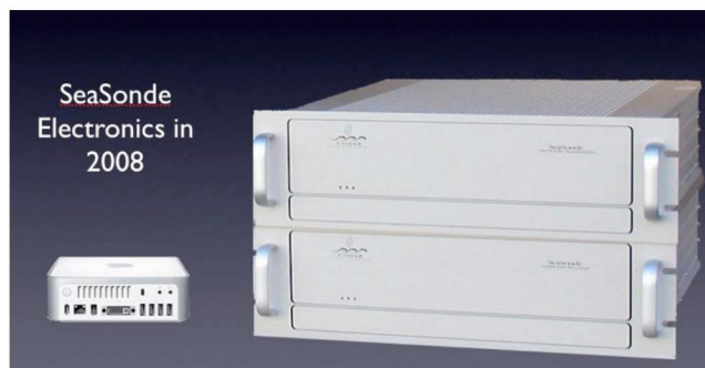
Figure 8. SeaSonde transmitter & receiver (right), and Mac Mini processor (left) as used in 2008.
