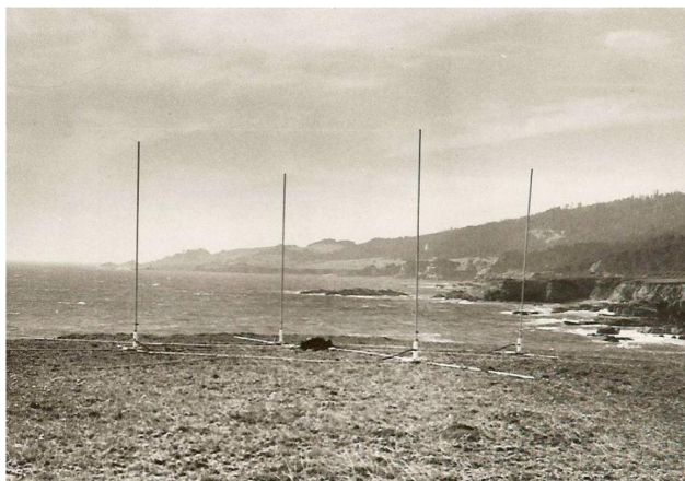
Figure 3. Photo of NOAA CODAR receive DF square array at 25 MHz.
