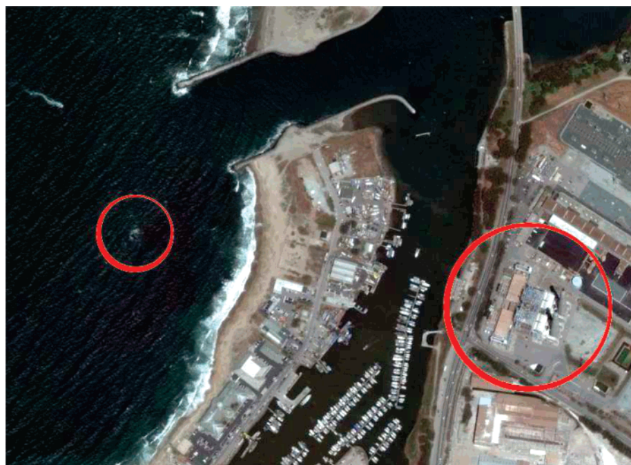
FIGURE 2. Aerial view of the Elkhorn Slough and the Duke power plant (right circle on the photograph). The plant exhausts warm water through a pipe that extends 200 m off the beach. The circle on the left of the photograph indicates the outlet of the pipe and the plume.
