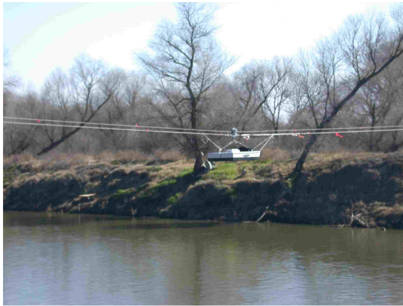
Figure 4. GPR antenna suspended over the San Joaquin River, California, on a light cableway system.
