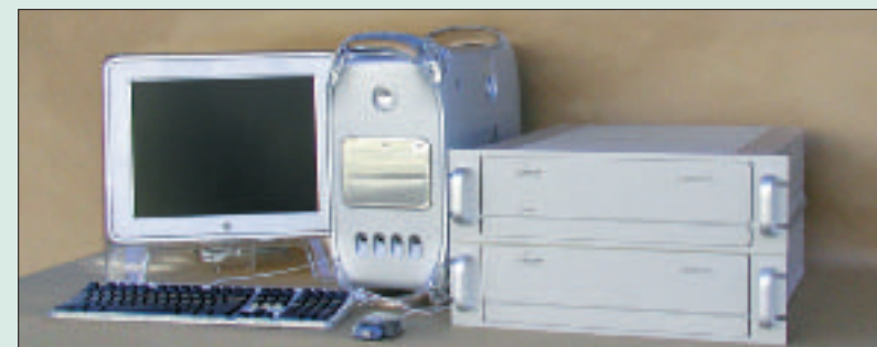
SeaSonde transmitter and receiver chassis with computer to control and process radar signals
