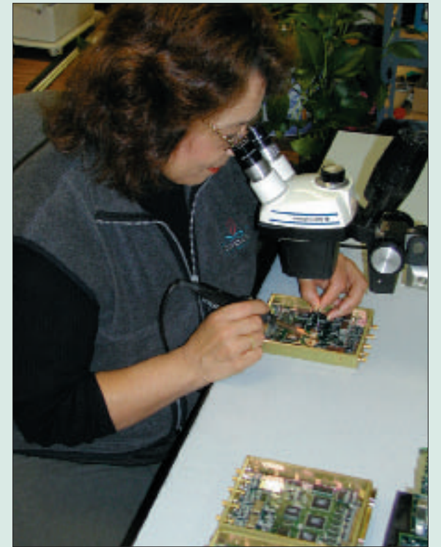
All system fabrication is done in-house, including these 6-layer circuit boards each requiring hundreds of solders
