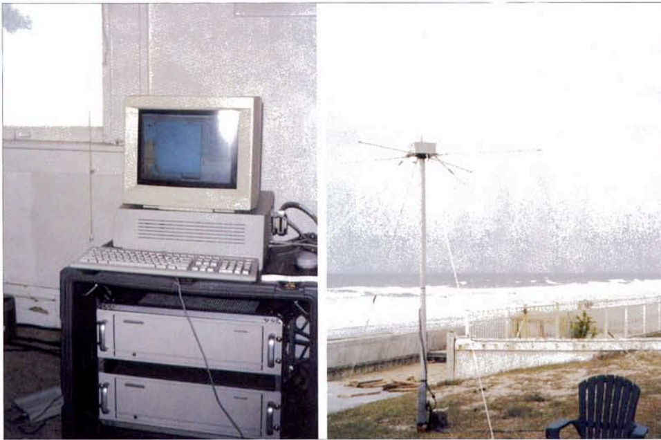
Figure 2: Photo of SeaSonde electronics (left) and antennas (right) at North site cottage
