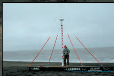
SeaSonde antennas have been striped with bright reflective tape for alerting snow machine operators to their presence.
