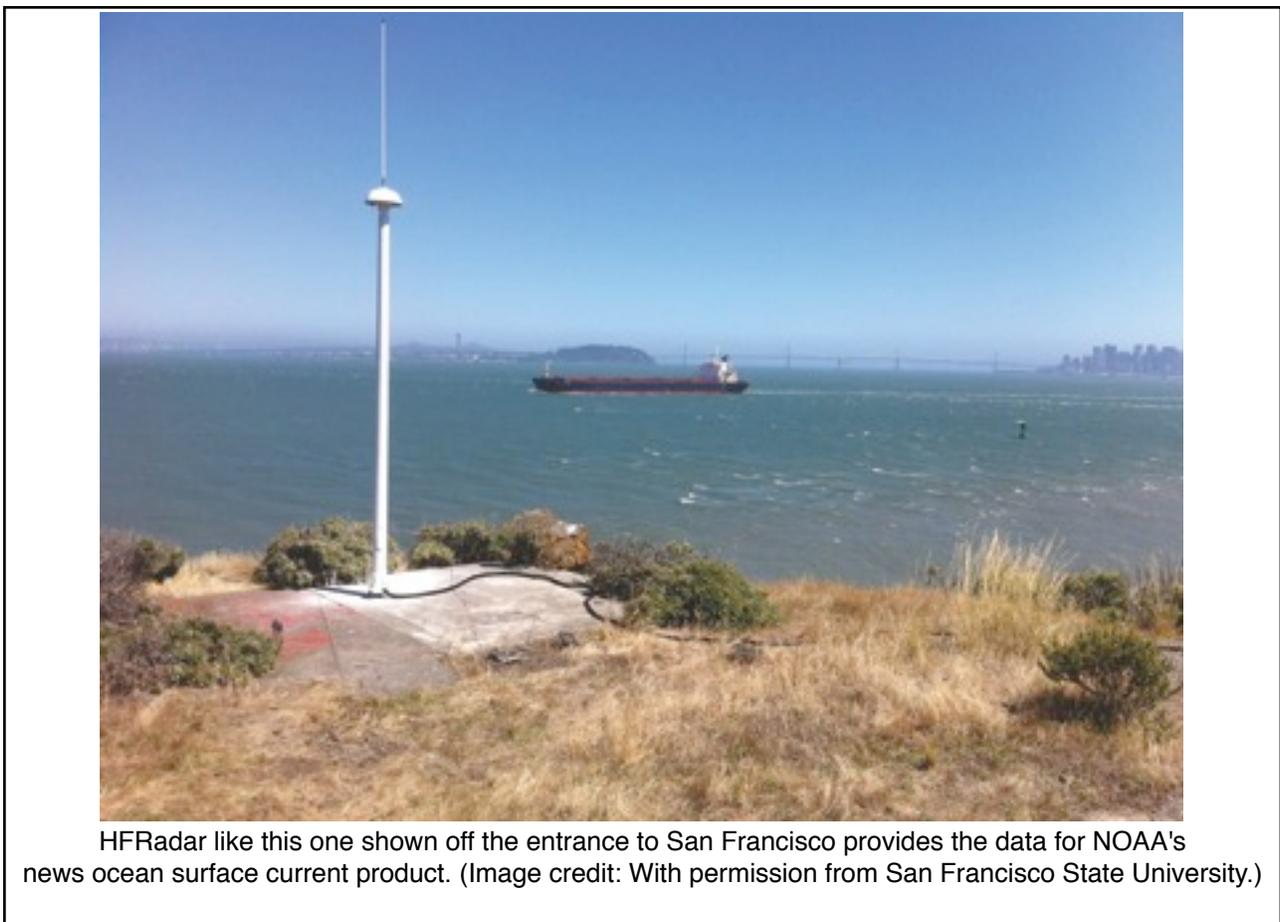
placed current measuring devices directly into the water to retrieve current speeds. While these direct measurement systems are still widely used as a standard reference, HF radars are the only sensors, including satellites, which can measure large areas at once with the detail required for important applications.
