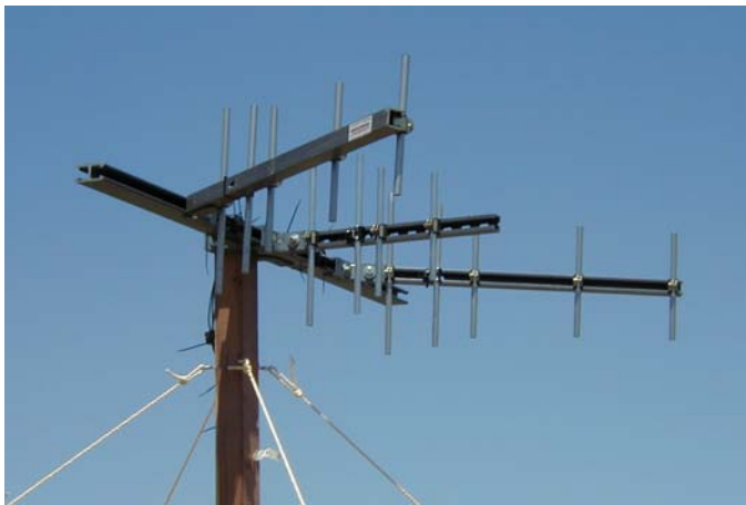
Fig. 3. Detail of the RiverSonde antennas. The middle antenna is used to illuminate a wide swath of water. Arrival directions of reflected signals are determined by processing signals received on all 3 yagis.
