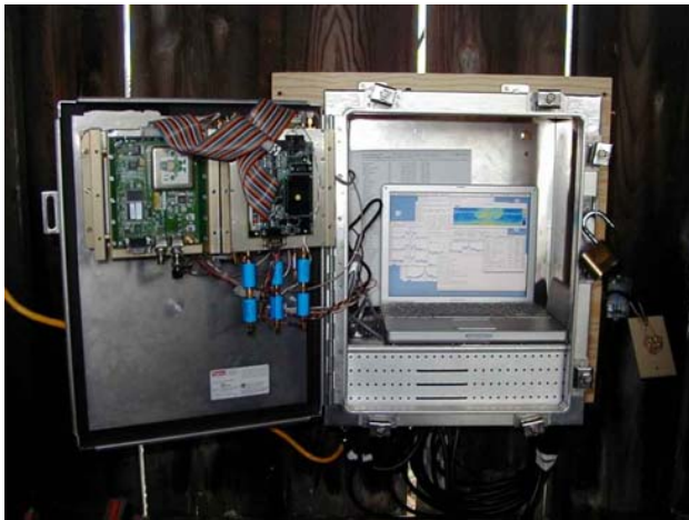
Fig. 2. RiverSonde equipment and laptop computer. The equipment is installed in a weather-resistant enclosure.
