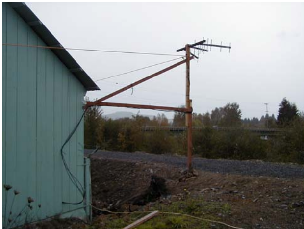
Fig. 3. RiverSonde antenna on the Cowlitz River at Castle Rock, Washington. Energy was transmitted on the center yagi and received on all 3 yagis.
