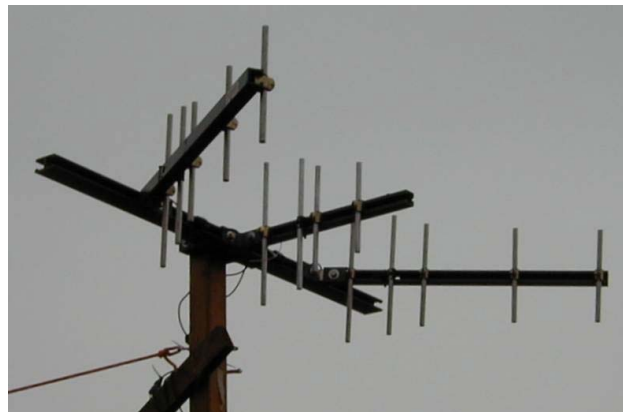
Fig. 1. RiverSonde antenna array. The spacing between the yagis is about 0.5 m.
