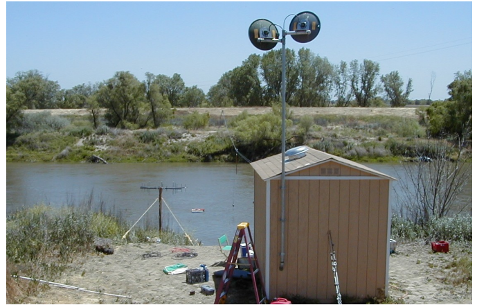
Fig. 2. Experimental setup at Vernalis, May, 2002. The RiverSonde antenna is on the near shore to the left of the building and receives signals from a wide angular sector, both upriver and downriver. Also visible are the narrow-beam microwave antennas above the building, and in-situ instrumentation in the water. Calibration of the RiverSonde antenna utilized a target carried by the cable across the river from the shelter to an anchor on the far bank.
