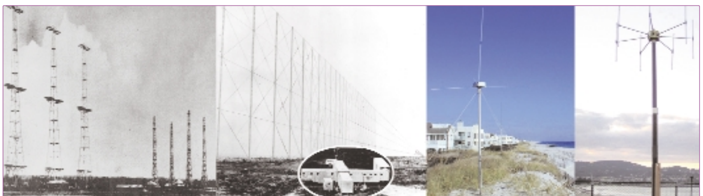
Figure 1. Evolution of HF receive antenna technology (from left to right) 'Chain Home' at English Channel, 1938; phased array on San Clemente Island 1972; commercial seaSonde®, 1999; compact superdirective receive array, 2003.
