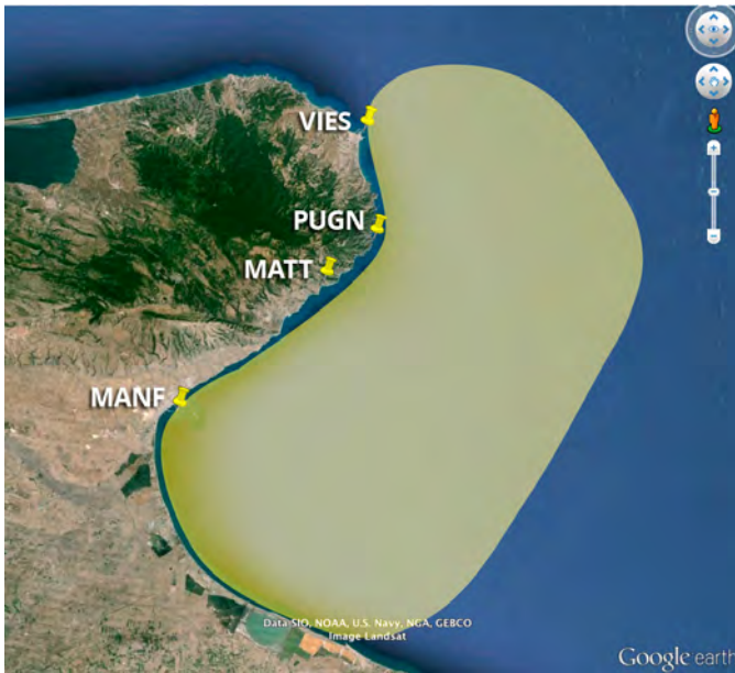
Fig. 1. Map of the ISMAR HF radar network node locations. The highlighted area indicates the coverage of the radar network.
