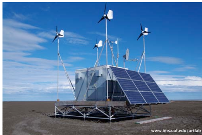
Figure 2: The remote power module (RPM) that powered the 25 MHz SeaSonde at Point Barrow.
