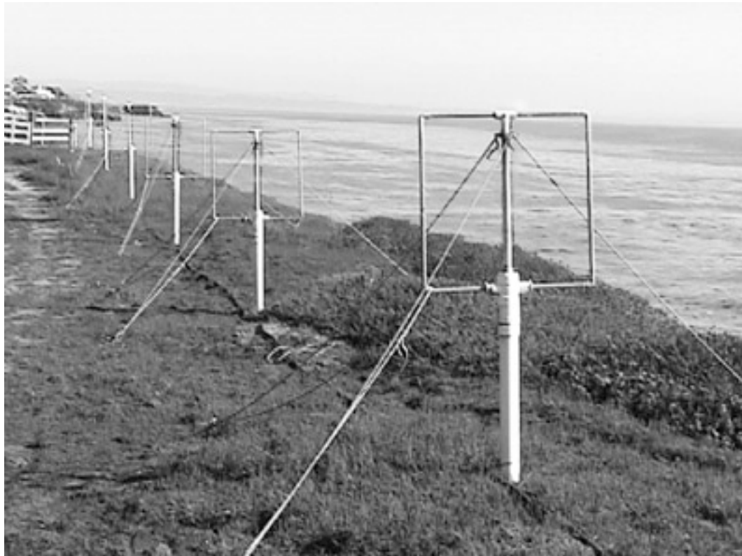
Figure 1.3: Loop elements of the MCR system's eight element receive array deployed at the Long Marine Laboratory site. The array pictured here is near the edge of a low bluff (about five meters above the sea surface) overlooking Monterey Bay.
