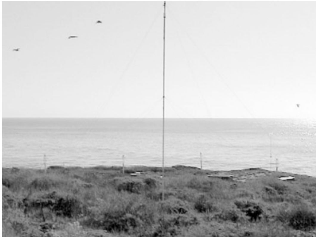
Figure 1.2: Location of the MCR system antennas at the Long Marine Laboratory deployment site showing the low frequency transmit antenna in the foreground and four of the eight elements in the receive array directly behind. The high frequency transmit antenna is not clearly visible in the photo but was located on a small point of land, on the ocean side of the receive array and toward the north end of the array (toward the right side of the photo). Pelicans in flight appear for scale to the left of the low frequency transmit antenna. Data from this system was the primary source for experiments discussed in this thesis.
