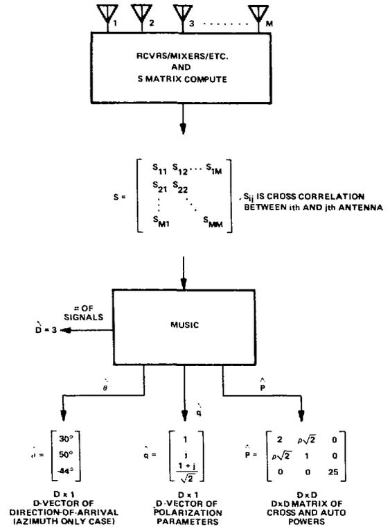
Fig. 2. Block diagram for multiple signal classification.
